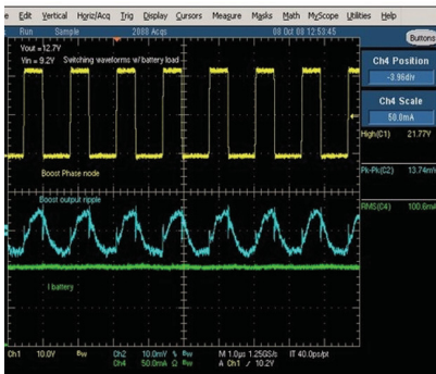
Figure 12 Typical converter waveforms highlight the battery load (top) and the boost output ripple current (bottom).
